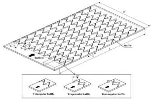
Fig4: Test section with rectangular, triangular, and trapezoidal baffles.
