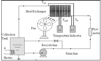
Fig. 2: Schematic of experimental setup [5]
